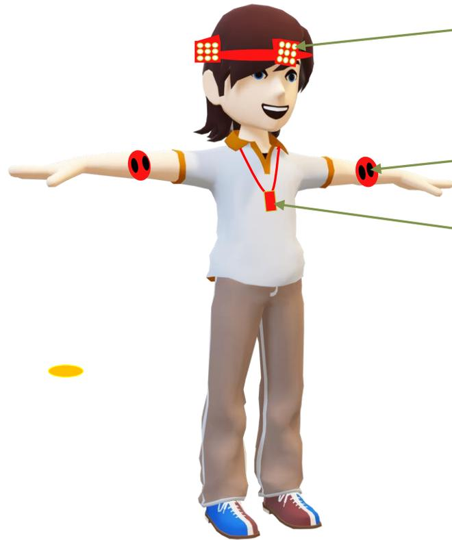
Down angled LED packs, double headband, front band carrying lights velcro-ed to cloth head band detachable for washing
